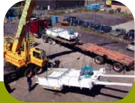
**Flextor offers a complete line of heavy-duty guillotine dampers to meet your requirements.** We have installed dampers in ducting sizes as large as 25' high by 16' wide. Our zero-leakage designs have been hydro-tested as high as 3 PSI and hydro tested at 60 PSI for structural integrity.
